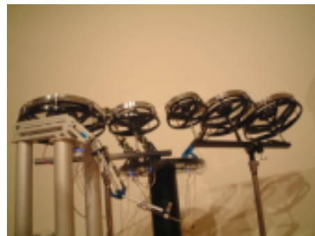
Fig.5: There is a special sort of springs in the arm of the robot. At the end of this, it holds a mallet.
