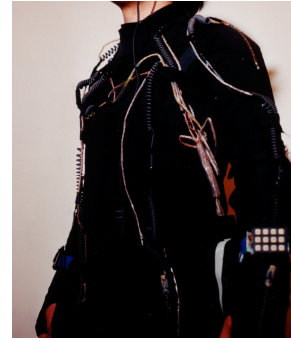
Fig.6: Upper half of body with “BodySuit.” The 12 bending sensors are placed on each joint of body.
