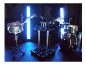
For this project, Suguru Goto developed his own robots with his original design, with collaboration with Fuminori Yamasaki, iXs Research Corporation (http://www.ixs.co.jp). Each robot, which is controlled by a computer in real time, represents a part of the human body and imitates the gesture of the human player.
